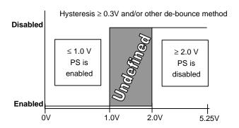
Figure 6: PSON# Signal Characteristics
